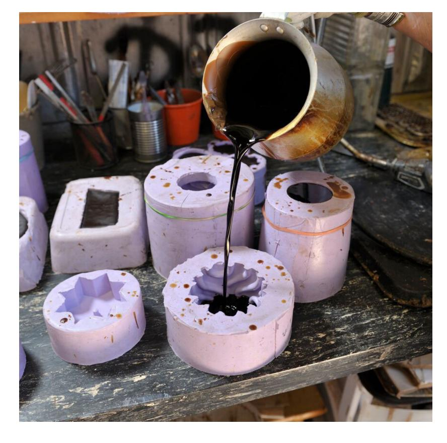
Lost wax casting is a versatile method that can be used to duplicate nearly any item as a glass object—that's right, that's right, we said nearly any item.
